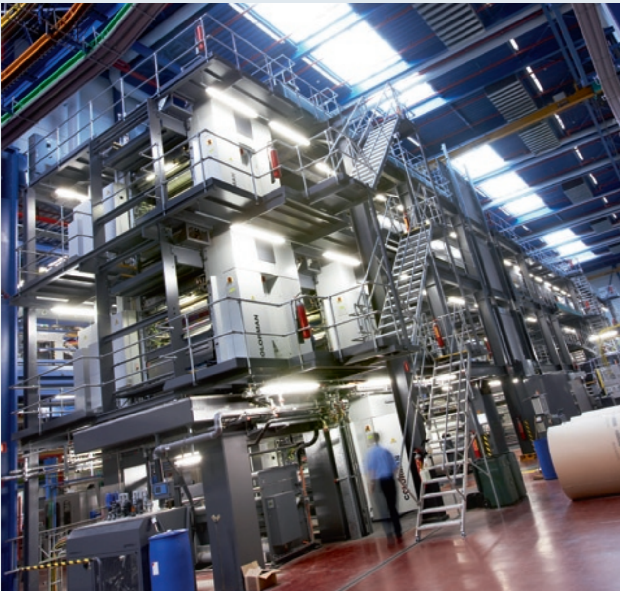
The world's largest heatset double-width newspaper press is installed at Roularta, Belgium. Each of the four Colorman 4-high towers is equipped with a horizontal MEGTEC dryer. The press has two quarterfolders to allow separate production of tabloid or broadsheet products. Source MAN Roland.
