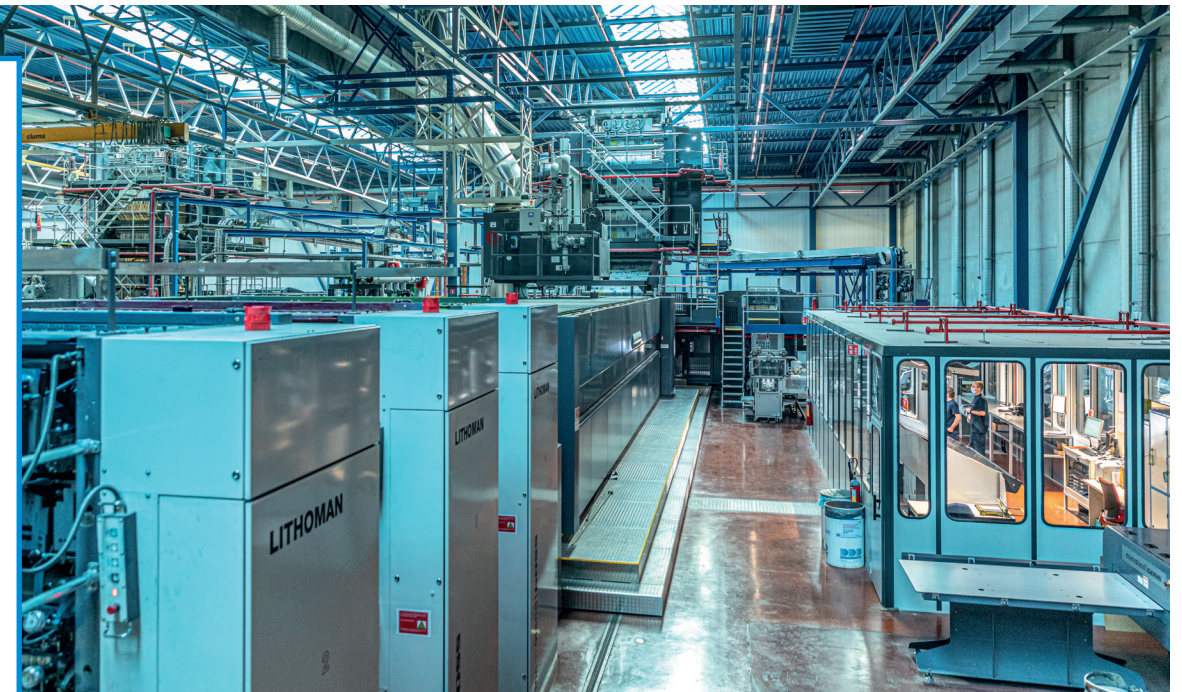
The new press can print 50,000 sections of 64 or even 72 pages each per hour.
